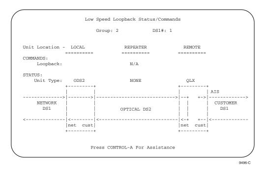
Figure 541-10b. Remote QLX Network Loopback Screen
